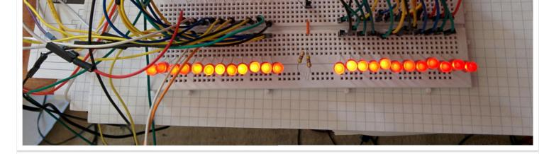
This is my test-bed. I connected up 46 LEDs (There are 48 GPIO pins on the BCM2835, but only 46 are brought out on the IO board – 46 isn't used and 47 is the new ACT LED on the IO board). The IO board is being powered via the main USB socket which is coming off a powered hub which also has a keyboard and Wi-Fi dongle connected to it.
